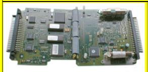
CENTRALINA DI GESTIONE MOTORE MSA15.5 INSTALLATA SULLE VETTURE BMW 318-325-525-725 TDS
